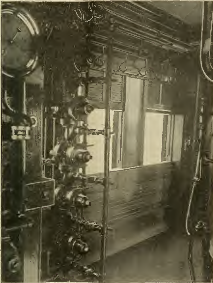
Fig. 2—TEXAS PACIFIC RY. AND INTERNATIONAL & GREAT NORTHERN R. R. INSTRUCTION CAR. DEFECTIVE TRIPLE VALVE RACK.
